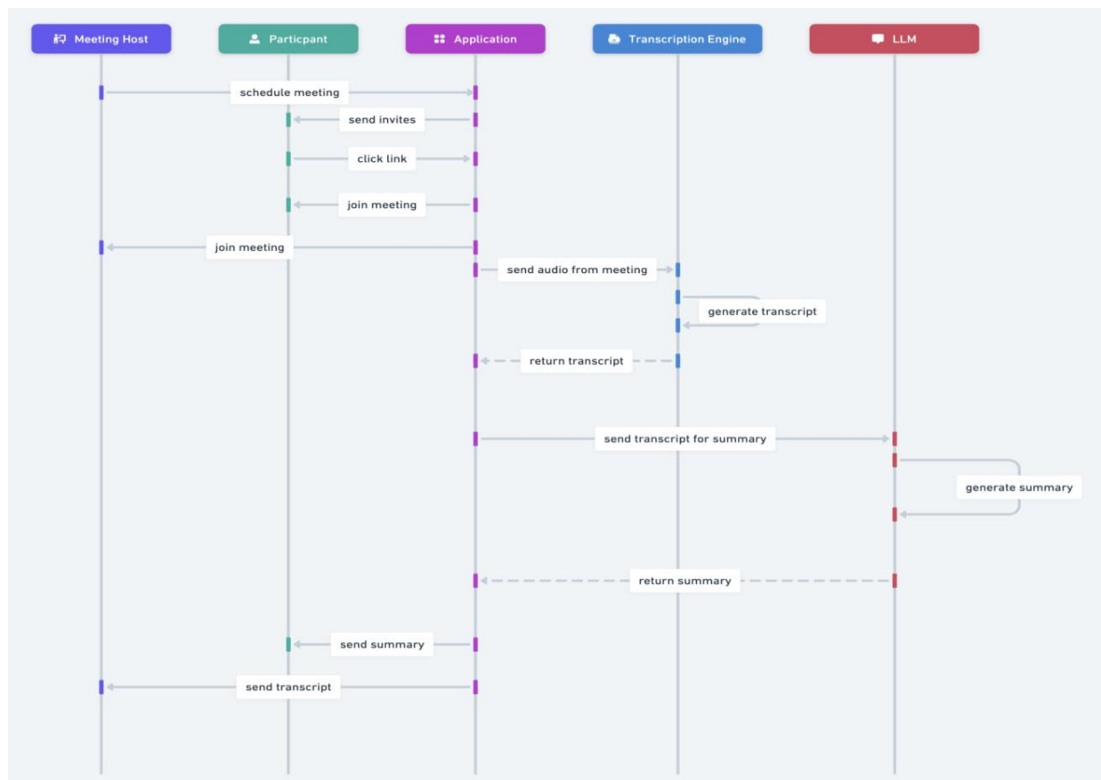
Figure 2: Sequence Diagram for Artificial Intelligence-Driven Video Conferencing Application
